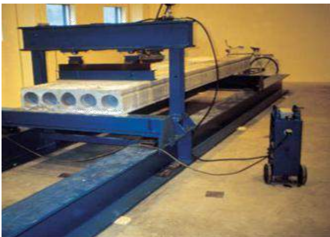
Shear test on hollow-core slab.
