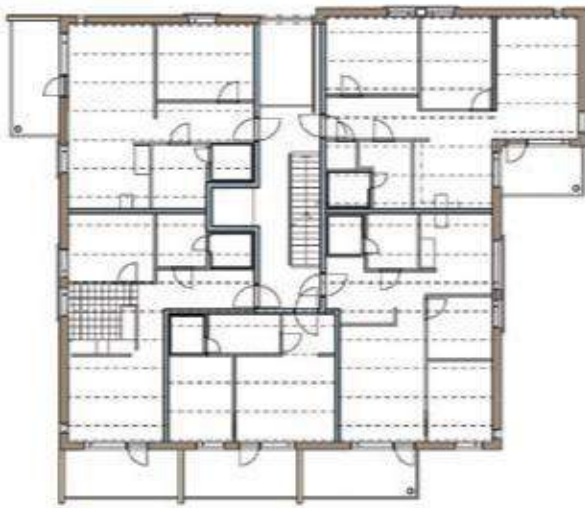
Layout of apartment building with load bearing façades and internal load-bearing cross-walls.
