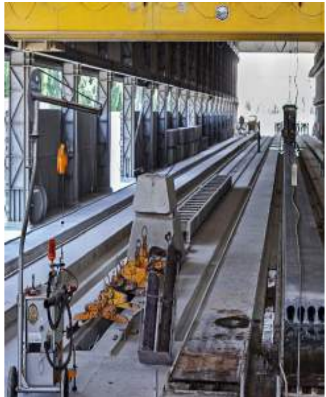
Hall for prefabrication of hollow-core slab.
