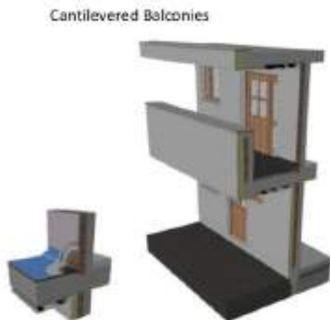
Cantilevering balconies with intermediate thermal insulation.
